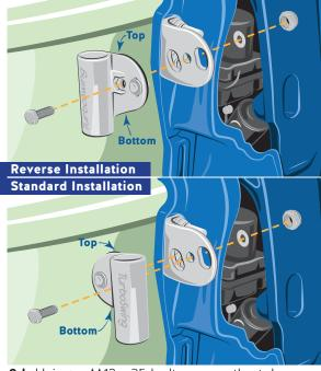
**2d.** Using a M12 x 35 bolt, secure the tube holder to the base plate and tighten using locking nut.
