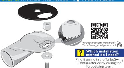
**2a.** Piece together the M8 x 25 bolt with the grooved locking nut onto the TurboSwing tube holder.
