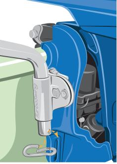
4. Complete your TurboSwing install by inserting the supplied carabiners into the holes at the bottom of the TurboSwing tube. If you are looking for a more permanent installation, feel free to replace the carabiner on either side with the supplied M8x45 bolts and M8 Lock Nuts.
