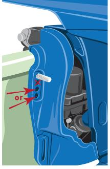
**1c.** Determine where to drill your TurboSwing holes using the base plate as a guide. Leave 1-2 holes in between the original and new bolts.
